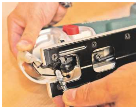
▲ You have to operate the lever to align the slot to allow the blade to slide in
